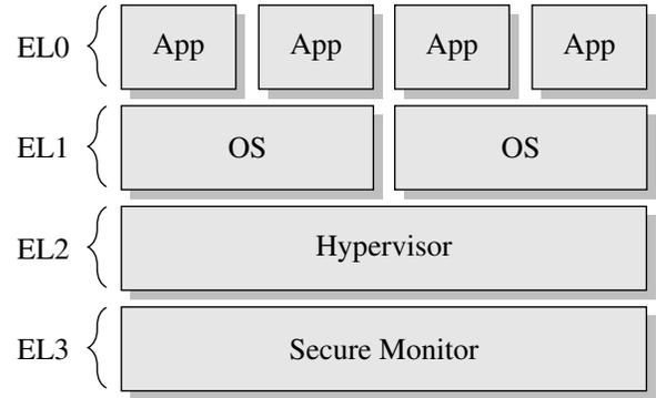
**Figure 1.** The ARM programming model. Moving down the exception levels increases privilege level. The secure exceptions levels are omitted for clarity.
