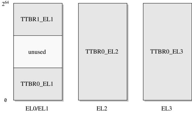
**Figure 2.** The ARM virtual memory model. EL0 and EL1 share an address space across two page table base registers, `TTBR0_EL1` and `TTBR1_EL1`. EL2 and EL3 have separate address spaces.
